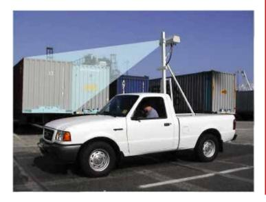
MIV is a simple, easy to use, and automated container inventory system that is catered for the operators to easily operate with a touch-screen computer while driving to perform the on-site containers checking at yards.
